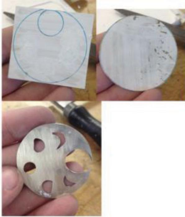
Figure 3. Three cutouts in silver, copper and brass.
